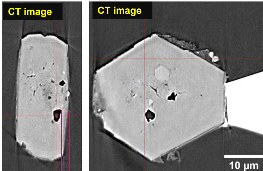
Depth from the sample surface to the inclusion (~2 μm)
