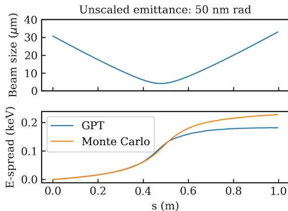
Figure 2: Beam size evolution (top) and slice energy spread growth (bottom) through a 1 m drift with 50 nm rad unscaled emittance.
