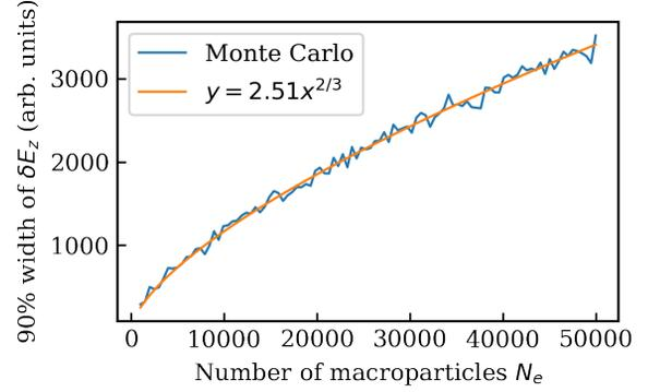
Figure 1: Scaling of the longitudinal space-charge field applied to each particle of the bunch. The width is computed at the RMS of a gaussian fit to the central 90% of energy kicks in the bunch.
