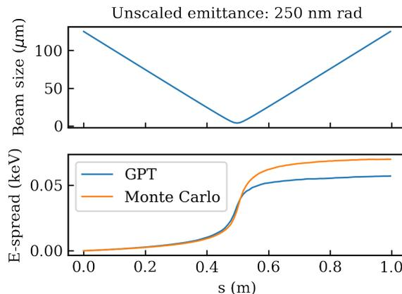
Figure 3: Beam size evolution (top) and slice energy spread growth (bottom) through a 1 m drift with 250 nm rad unscaled emittance.
