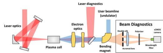
Figure 5: Schematic layout of the interferometry beam size monitor (IBSM) for a plasma-wakefield accelerator.
