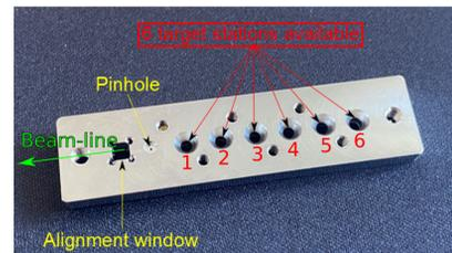
Figure 6: Picture of the sample holder for static diffraction experiments.
