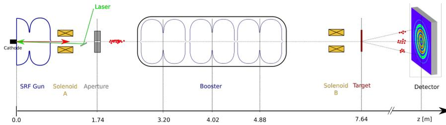
Figure 1: Sketch of the SRF Photoinjector beam-line with UED related components.
