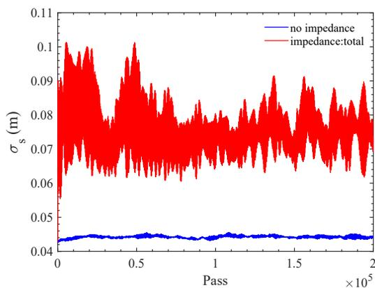
Figure 3: The impedance effects to an electron bunch length in the SPS storage ring.
