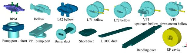
Figure 1: The 3G geometries of vacuum components of the SPS storage ring (not to scale).
