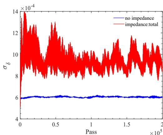
Figure 4: The impedance effects to an electron beam energy spread in the SPS storage ring.
