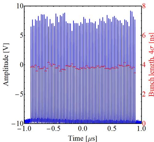
Figure 4: Typical bunch profile of the last turn in the PS (blue) and  $4\sigma$ -bunch length (Gaussian fit) of the 72 bunches at an average intensity of  $2.8 \cdot 10^{11}$  p/b (2021 data).
