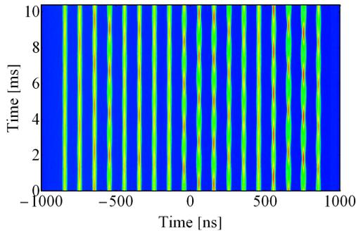
Figure 3: Quadrupolar coupled-bunch instabilities evolving at the flat-top (2021 data). The dominant mode number,  $n = 4$  with a bunch-by-bunch phase advance of  $\Delta \phi_{bb} = 4 \times 2\pi/18$ , is identical to the one observed before LS2.
