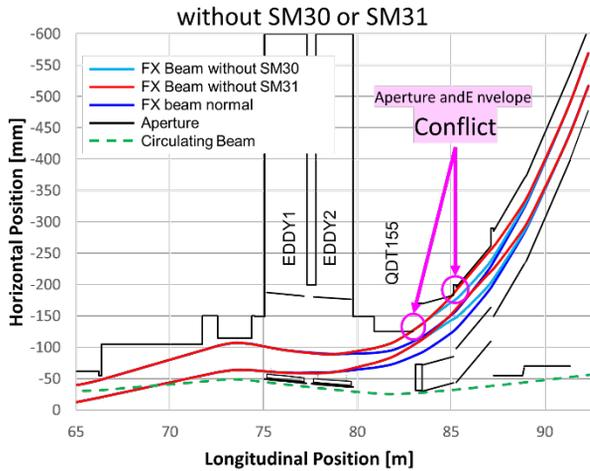
Figure 4: Failure cases of the SM30 or SM31.
