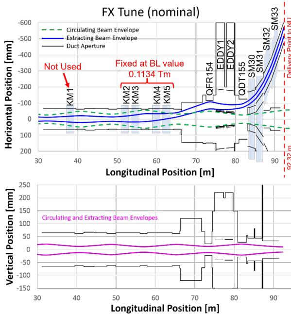
Figure 2: FX tune beam envelopes.
