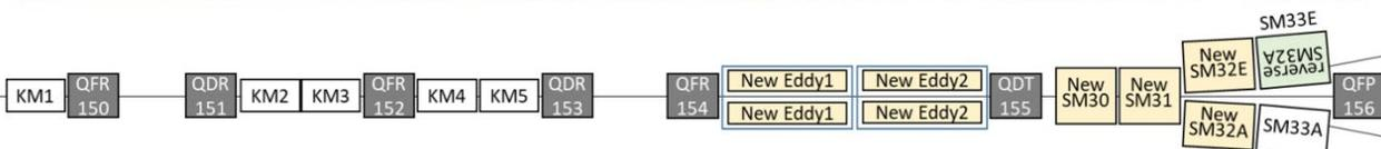
Figure 1: The layout of the FX magnets at J-PARC MR.
