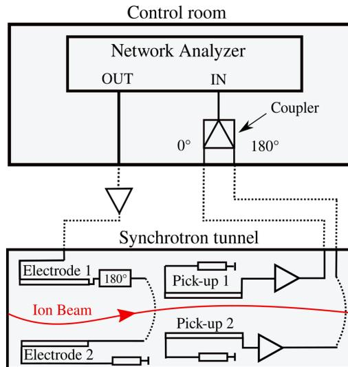
Figure 1: BTF experimental setup. The network analyzer (NA) generates an excitation signal and scans over a frequency span of interest. The response of the beam is then measured with two pick-up electrodes.
