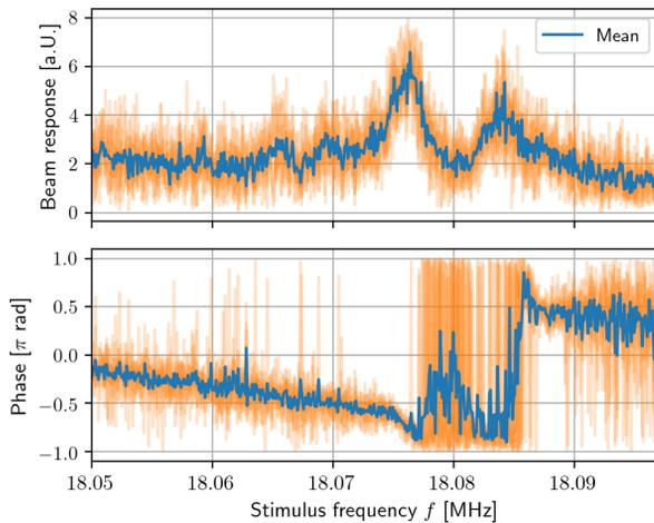
Figure 2: Measured horizontal beam response at extraction conditions. Orange background: Overlap of eight different shots. Blue solid curve: Mean value of the eight recorded shots.
