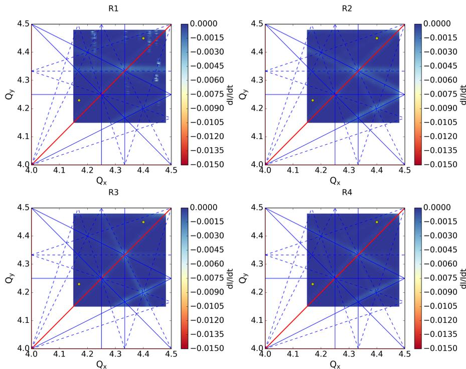
Figure 2: Loss maps resulting from dynamic tune scans in all four rings of the PSB with octupoles and sextupoles for the simultaneous correction of the 3<sup>rd</sup> and 4<sup>th</sup> order resonances. The color coding and the resonance lines are as in Fig. 1. The yellow points correspond to the tune ramp used in the optimization framework.
