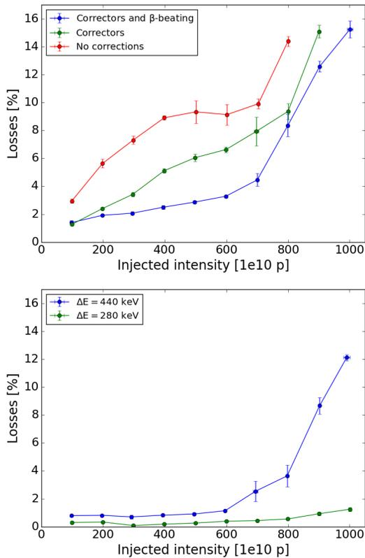
Figure 3: Total losses for the ISOLDE user versus the injected intensity for an injection working point of  $Q_x, Q_y = (4.22, 4.45)$  (top) and  $Q_x, Q_y = (4.22, 4.35)$  (bottom). The losses are calculated with or without resonance compensation and including the  $\beta$ -beating corrections [2] (top) and different energy spread (bottom).
