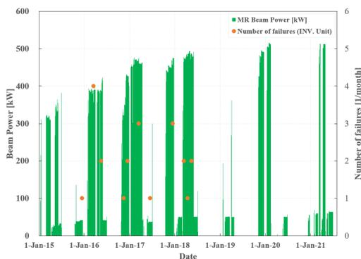
Figure 5: History of MR beam power and number of failures (inverter units) since 2015.
