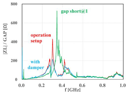
Figure 4: The impedance of a 4-gap cavity measured by the stretched wire method. Resonant modes exist in the region of several hundred MHz regardless of conditions.
