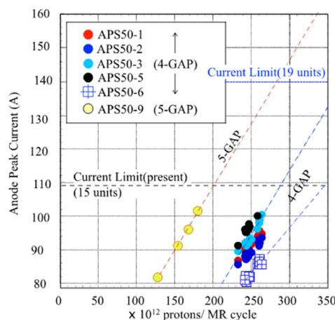
Figure 1: The measured peak anode current of the APS versus the number of circulating protons.
