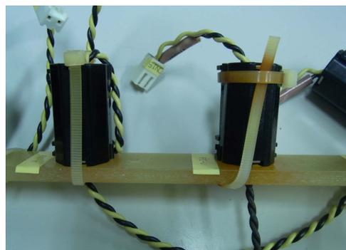
Figure 6: A noise filter in the failed inverter unit.
