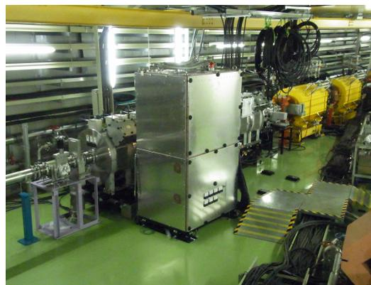
Figure 3: Two 2<sup>nd</sup> harmonic RF cavities with FT3M. The first of the 2<sup>nd</sup> harmonic RF cavity is ready for operation. The second one, the cavity was installed and a final stage amplifier will be connected in 2023.
