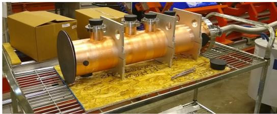
(b) The outer tube sub-assembly being leak-checked after the ports were brazed.
