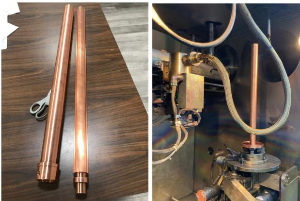
(a) The center conductor CNC-machined for multiple tapering. (b) The center conductor sub-assembly in the welding chamber.
