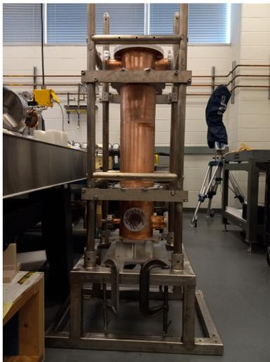
Figure 5: The kicker cavity placed in the cage for the bench test. Its orientation is upside down for measurement convenience.
