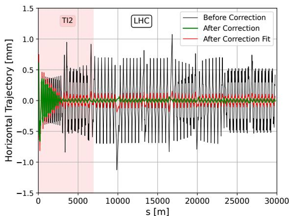
Figure 5: Transfer line trajectory and LHC injection oscillations induced by an orbit drift in the SPS (black line). The results of the steering performed based on the actual  $x$  and  $x'$  values at extraction (green line) and those obtained with the fitting curves are also plotted.
