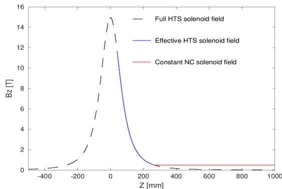
Figure 2: On-axis field of the HTS solenoid. A small part of the constant NC solenoid field is also displayed.
