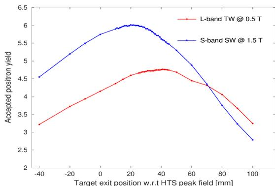
Figure 4: Scan of Accepted Positron Yield as a Function of the Target Exit Position
