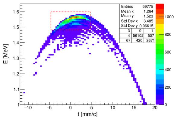
Figure 3: Longitudinal phase space of the positrons at the end of the injector linac for the L-band TW structures capture linac profile. Energy and time cut window are displayed by a red dashed rectangle on the plot. The time of the reference particle is set to 0.
