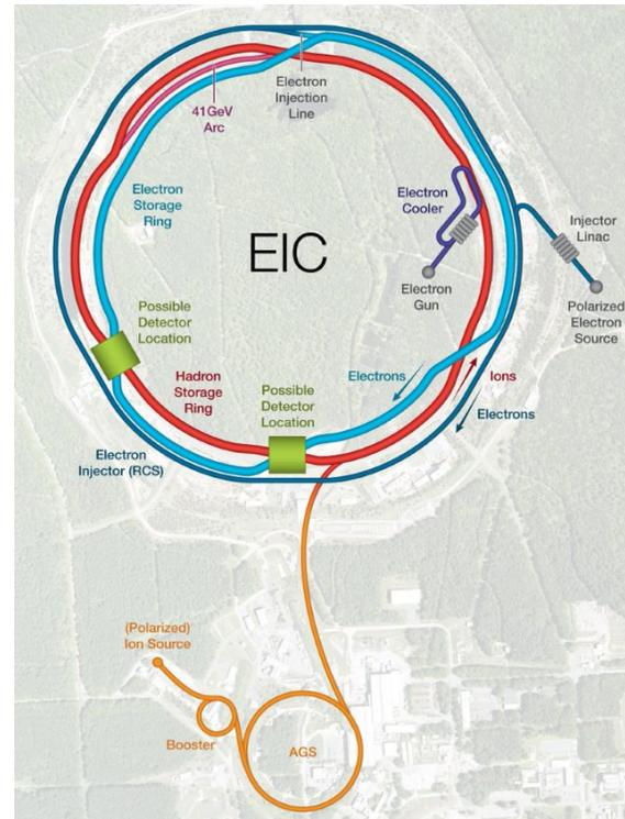
Figure 1: Schematic diagram of the EIC complex.
