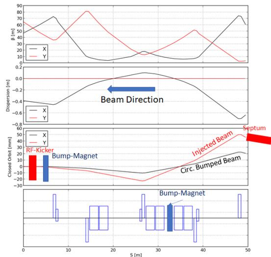
Figure 4: Circulating and injected beam trajectories in RCS.
