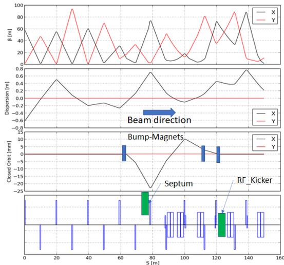
Figure 3: Beam parameters and bump, of injection section.
