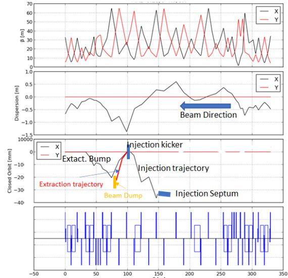
Figure 7: Parameters/trajectory at ESR injection region.
