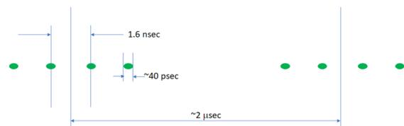
Figure 2: Bunch pattern at RCS injection.
