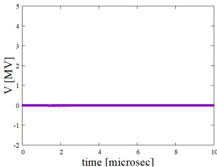
Figure 4: Imaginary part of the cavity voltage evolution with 22.5 MW RF power with 1 A beam loading current starting at the filling time. PM with no delay is applied.
