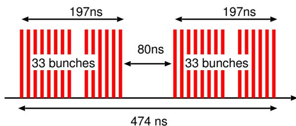
Figure 1: The beam structure in the positron source. Each mini-train contains 33 bunches. Each pulses contain 2 or 1 mini-trains.
