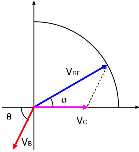
Figure 2: Phase diagram of  $V_{RF}$  (blue arrow),  $V_B$  (red arrow), and  $V_C$ . PM angle  $\phi$  should determined as the  $V_{RF}e^{i\phi} + V_Be^{i\theta} = V_C$
