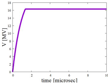
Figure 3: Real part of the cavity voltage evolution with 22.5 MW RF power with 1 A beam loading current starting at the filling time. PM with no delay is applied.
