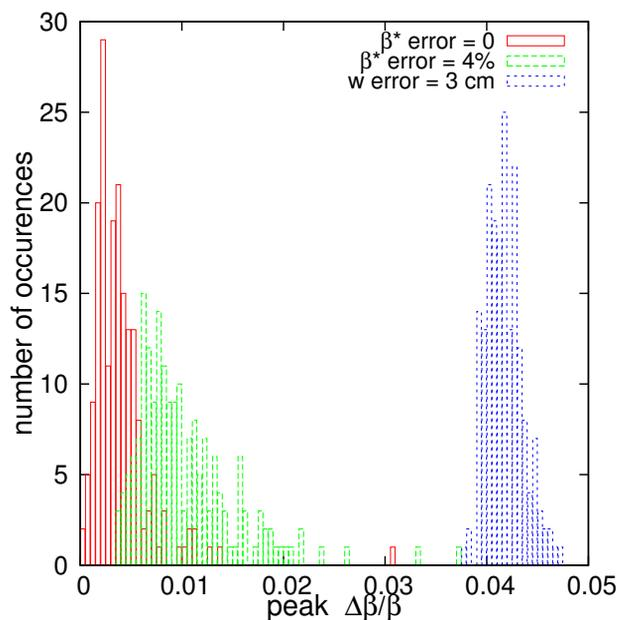
Figure 2: Peak residual  $\beta$ -beating after applying APJ corrections to 200 different IR error distributions. Three different histograms are shown: with no error in  $\beta^*$  (red), with a 4% error in  $\beta^*$  (green) and, with 3 cm error in  $w$  (blue).
