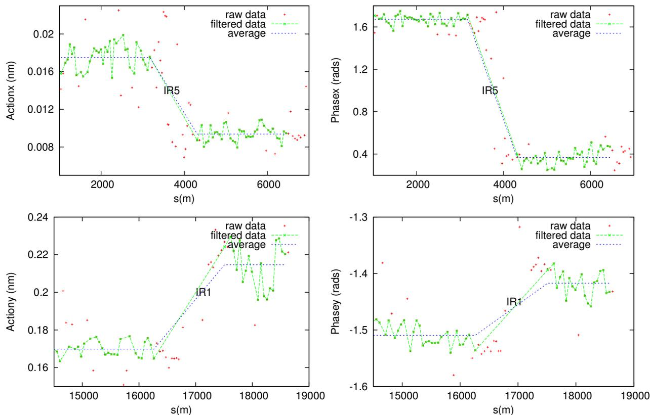
Figure 1: Action and phase plots around IR5 for beam 2 (top) and action and phase plots around IR1 for beam 1 (bottom). Average values in the arcs (blue horizontal lines) and in the inter-triplet spaces (no shown) are used to estimate the corrections.
