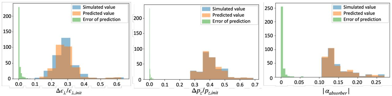
Figure 2: Random Forest model prediction compared to the tracking simulation of transverse emittance reduction, longitudinal momentum reduction and Twiss parameter  $\alpha$  in the absorber regions. Prediction errors are computed as absolute difference between true simulated and predicted values.
