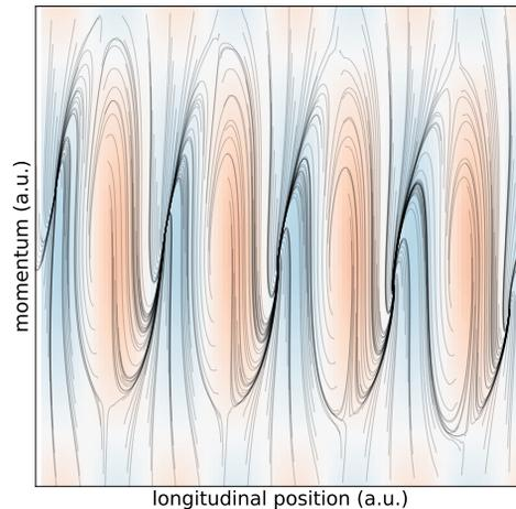
Figure 3: Attractor plot example. The blue and red regions show the relative cooling/heating force of every point in phase space integrated over a single synchrotron period. The black lines track the evolution of particles undergoing the single-pass shaping scheme.
