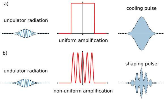
Figure 2: Conventional (a) and non-uniform (b) undulator-radiation amplification.
