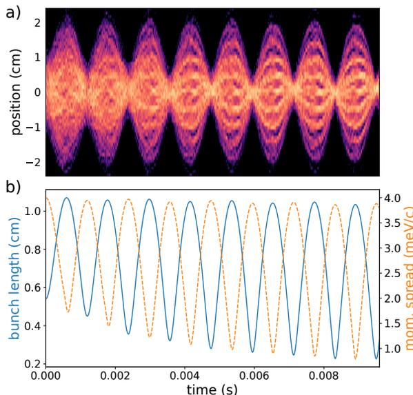
Figure 5: Demonstration of microbunch formation. Waterfall plot of the evolution of the longitudinal bunch distribution (top), and corresponding rms bunch length and energy-spread evolution over 10 ms (bottom).
