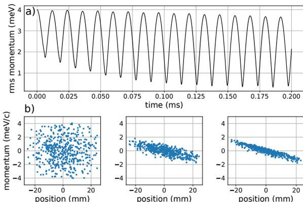
Figure 4: Energy spread reduction using multipass gain modulation. The top plot shows the r.m.s. momentum spread. The lower plots are the LPS distributions at synchrotron periods 1, 8, and 17.
