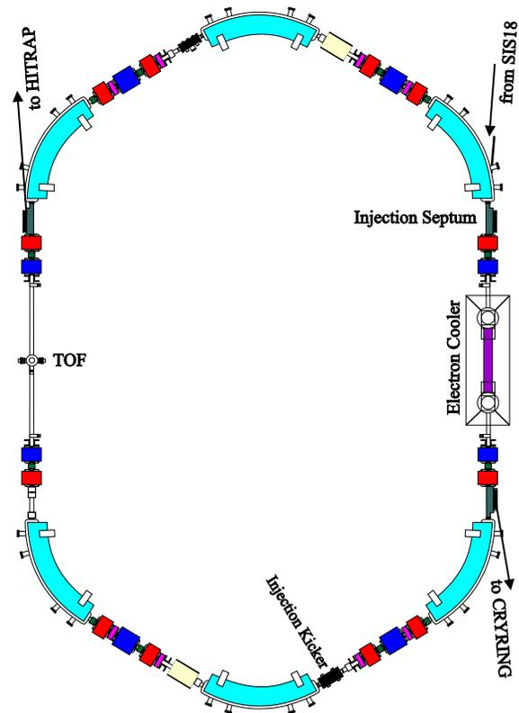
Figure 1: Layout of the Experimental Storage Ring (ESR). Dipoles, focusing, defocusing quadrupoles and sextupoles are marked by light blue, red, blue and pink colors correspondingly. Positions of the electron-cooler and the TOF detector are indicated in the straight sections.
