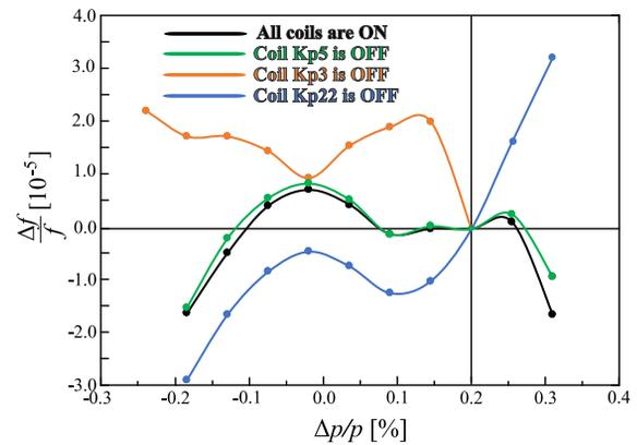
Figure 3: The effect of most powerful dipole correction coils on the isochronicity. The injection orbit  $\Delta p/p = +0.2\%$  has been chosen as a starting point for the measurements. The sextupole setting was not applied.
