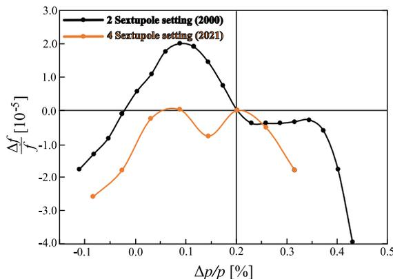
Figure 4: The isochronicity curves corresponding to the different settings using 2 sextupole families (black curve) and 4 of them (red curve). The injection orbit  $\Delta p/p = +0.2\%$  has been chosen as a starting point for the measurements.
