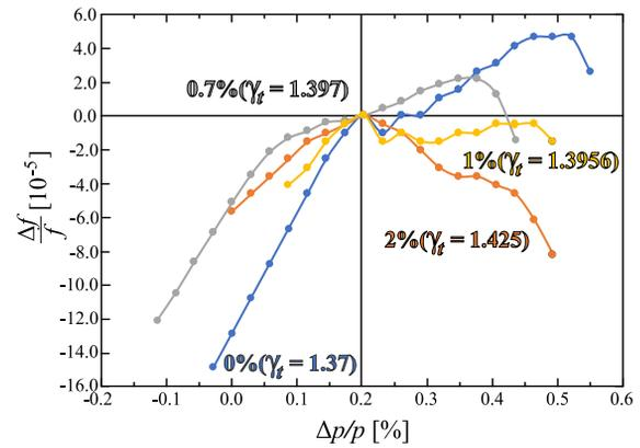
Figure 2: The isochronicity curves corresponding to the different strengths of one defocusing quadrupole family GE01QS3D of the ESR. The strength of 1% higher than default one shows a good agreement of  $\gamma_t = 1.3956$  with a beam  $\gamma$ . The injection orbit  $\Delta p/p = +0.2\%$  has been chosen as a starting point for the measurements. The sextupole setting was not applied.
