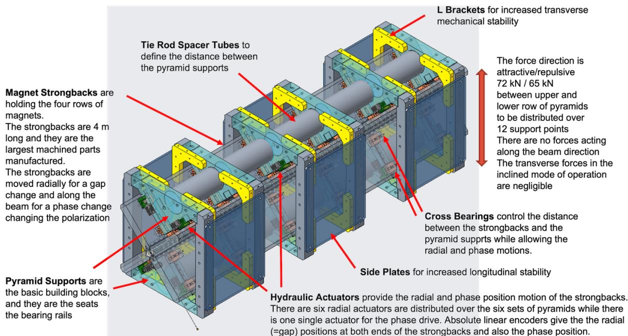
Figure 1: Overview of the mechanical system of the 4 m long LBL X-type undulator.
