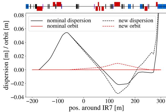
Figure 3: Comparison of the single pass dispersion starting at the primary collimators for the nominal case (solid lines) and the orbit bump (dashed lines).
