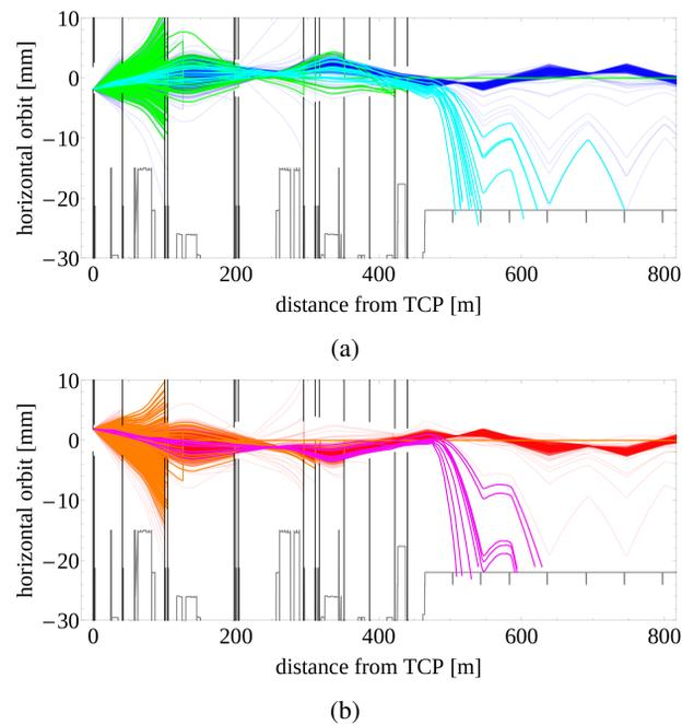
Figure 2: Tracks of particles scattered out of the horizontal primary collimator jaws, (a) for negative jaw and (b) for positive jaw. Blue/Red particles survive, Green/Orange particles would be lost in the DS if not for the secondary collimators, Cyan/Magenta particles leak out and are lost in the DS. Black lines are collimators and grey are the aperture.
