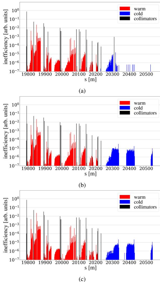
Figure 1: Example loss maps zoomed into IR7 for a few cases. (a) is for relaxed settings including the TCLD at  $\beta^*=20$  cm, (b) excludes the TCLD and (c) has a dispersive orbit bump and TCLAs offset by  $3\sigma$ .
