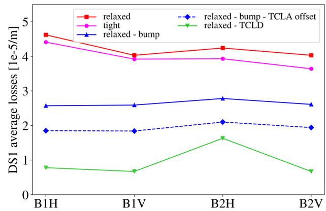
Figure 4: Comparison of the average losses in the first DS cluster for the different scenarios. B1(2) refers to beam 1(2), while H refers to horizontal and V to vertical loss maps.
