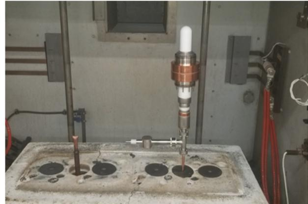
Figure 1: The prototype 1497 MHz magnetron in the bakeout oven at RELL, showing the ion pump used for conditioning.
