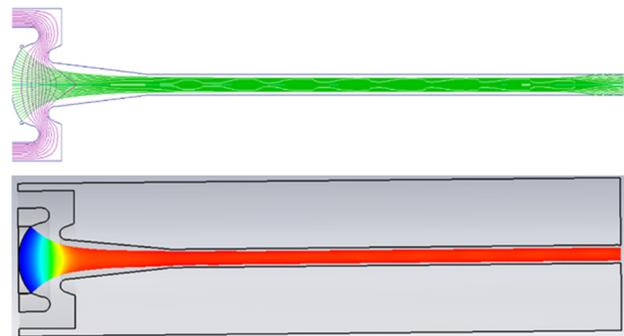
Figure 5: Beam optic simulation result in DGUN and CST.
