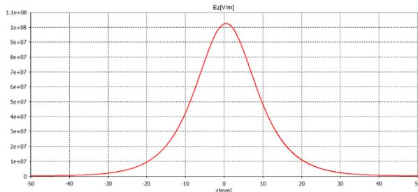
Figure 3: The electric field on z axis around a second harmonic cavity.
