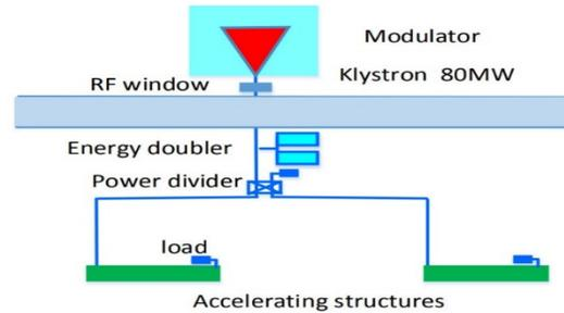
Figure 1: Accelerating structure of CEPC LINAC.
