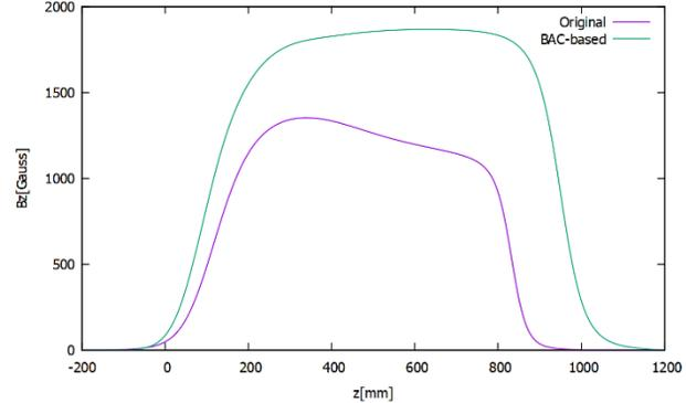
Figure 4: Comparison of the magnetic field on z axis.
