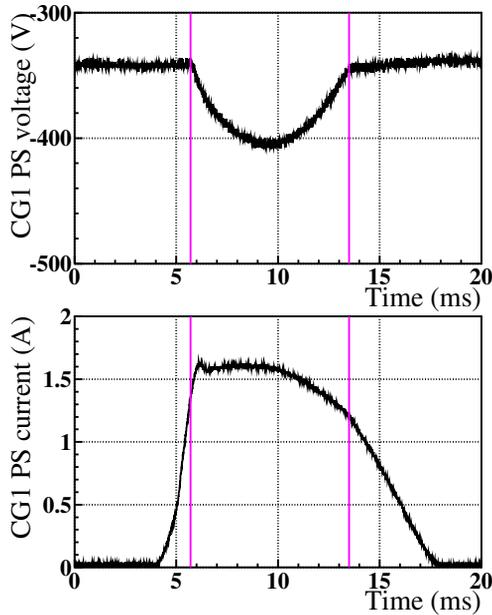
Figure 4: Control-grid DC-bias voltage drop and control-grid current.
