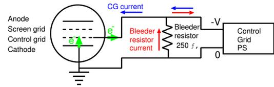
Figure 5: Current flows provided by the control grid power supply and the tube.
