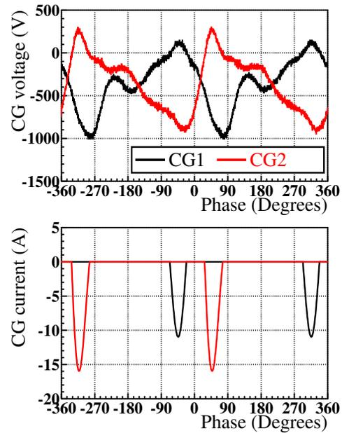
Figure 3: The measured waveform of the control grid voltage and the estimated control grid current.
