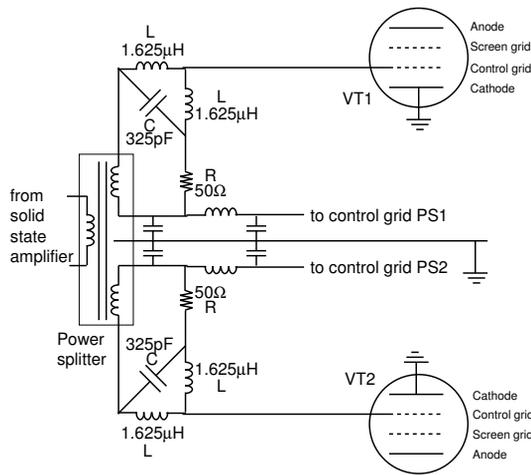
Figure 1: Schematic view of the control grid circuit.
