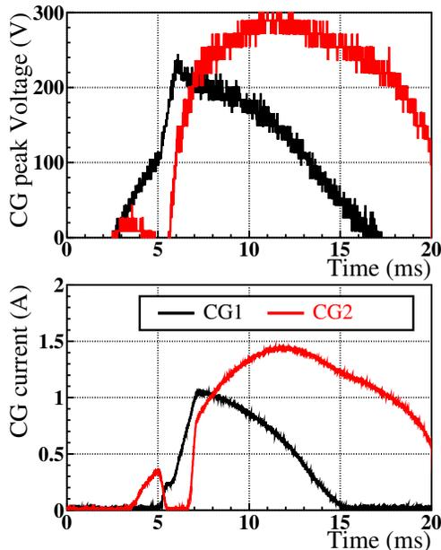
Figure 2: The measured results of the control grid peak voltage and control grid current.
