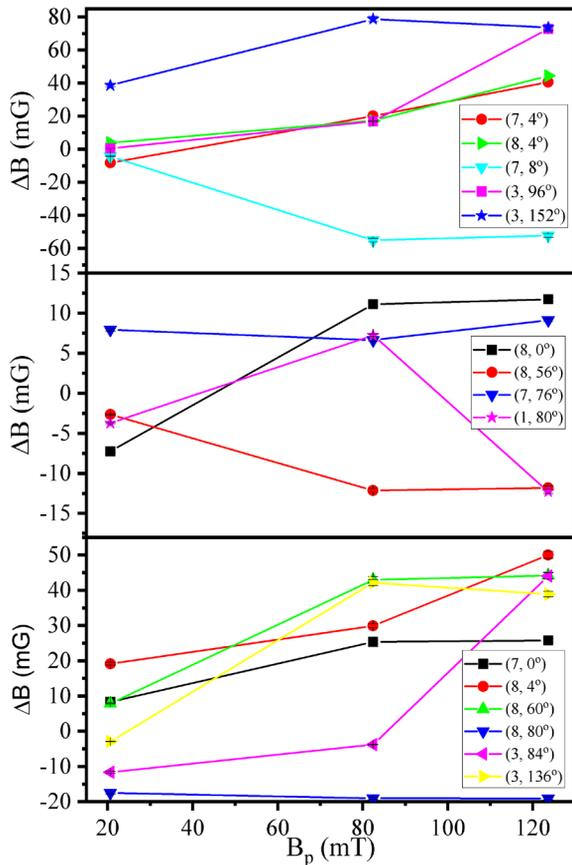
Figure 4: Change in the magnetic field ( $\Delta B$ ) measured by Hall Probes (top plot), AMR radial (middle plot), and AMR tangential (bottom plot) sensors versus  $B_p$  at selected locations, identified by the pair (sensor number,  $\theta$ ).
