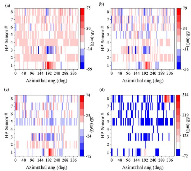
Figure 6: Change in radial magnetic field  $\Delta B$  measured by Hall probes versus azimuthal angle  $\theta$  measured at (a) 5 MV/m, (b) 20 MV/m, (c) 30 MV/m, and (d) zero RF power after the quench. The measurements were made at 2 K after a slow cool-down in an applied field of  $\sim 115$  mG.
