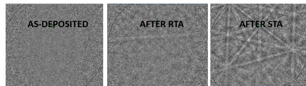
Figure 6: Electron diffraction patterns (Kikuchi lines) for as-deposited, after RTA, and after STA samples, where one can clearly see no signal for the as-deposited ones, a weak signal for the RTA samples, and a remarkable signal for the STA samples.
