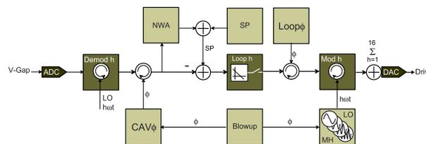
Figure 1: Building blocks of the multi-harmonic digital feedback system implemented in FPGA. Demodulator, feedback loop and modulator blocks are replicated 16 times.
