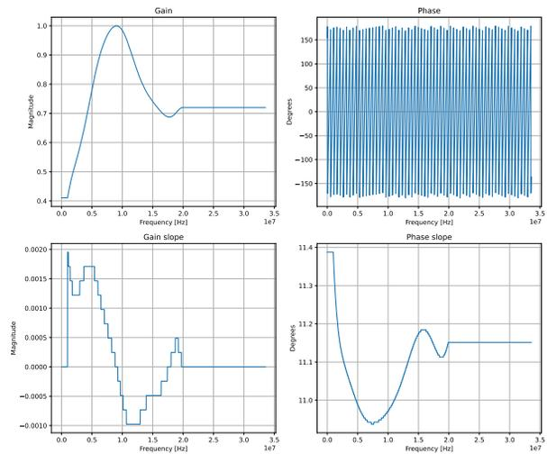
Figure 2: Example of the values of an operational feed-forward compensation table. The gain and phase compensation values are computed for different frequency values. The slope values are used for interpolating the actual gain and phase corrections.
