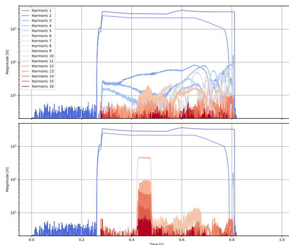
Figure 4: Detected voltage of one cavity when enabling only harmonic 1 and 2 feedback loops (upper figure) or 16 loops (lower figure). When all loops are enabled the blow-up phase noise contribution can be observed in harmonic 10. The beam intensity during this measurement was about  $95 \cdot 10^{10}$  protons per bunch.
