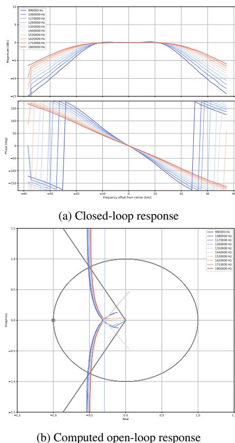
Figure 3: Embedded network analyzer acquisition and computation of open-loop response. The average gain margin is 10.24 dB whereas the average phase margin is 60.10 degrees.
