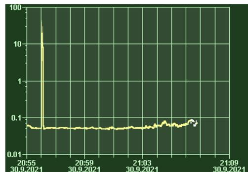
Figure 7: LLRF system vector sum phase regulation performance (dP in [deg]) in time.
