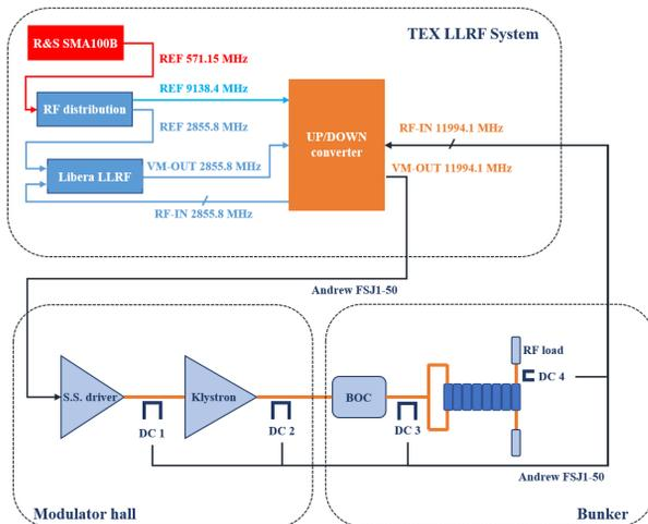
Figure 3: TEX RF system block diagram. It includes also the BOC pulse compressor that will be added in a second phase.
