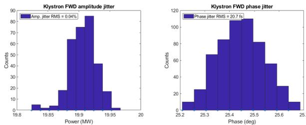
Figure 5: Measured amplitude and phase jitter of klystron output forward power. The measurements refer to 20 MW, 300 ns at 50 Hz repetition rate RF pulses.
