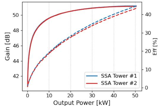
Figure 1: Sirius RF SSAs efficiency (dashed) and gain (solid).
