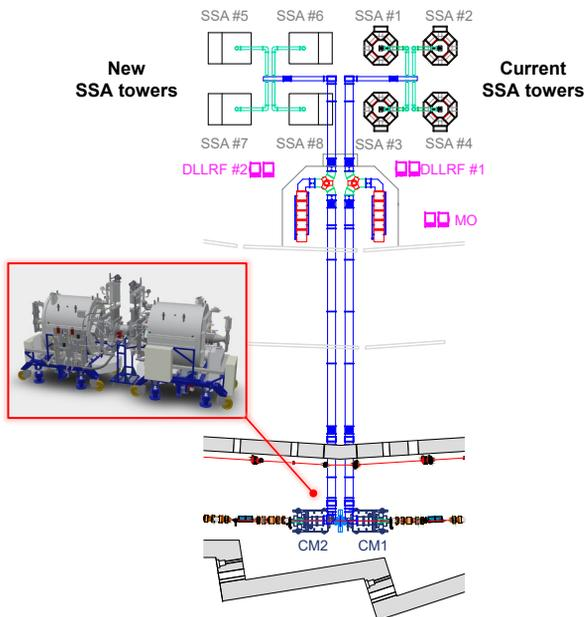
Figure 6: Layout of the RF system for the SC cavities.
