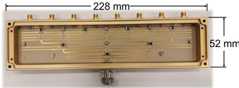
Figure 2: Top view of the 8-way divider prototype.
