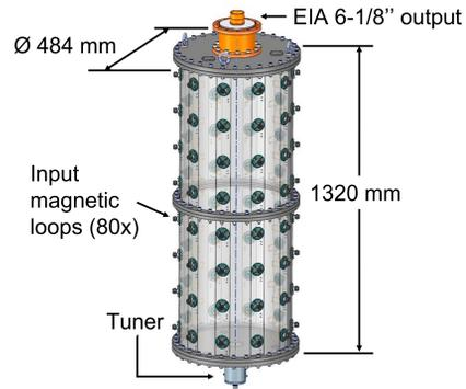
Figure 6: View of the proposed cavity combiner 3D CAD.
