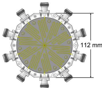
Figure 3: View of the 10-way divider mechanical CAD.
