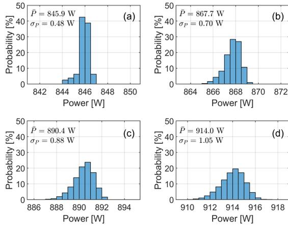
Figure 5: Maximum incident power for (a) 1, (b) 2, (c) 3 and (d) 4 faulty modules on random input ports.
