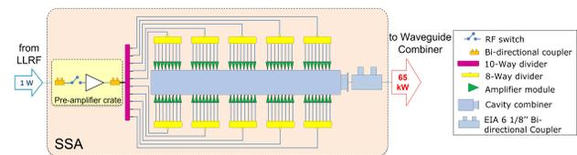
Figure 7: Schematic of the SSA's RF system.
