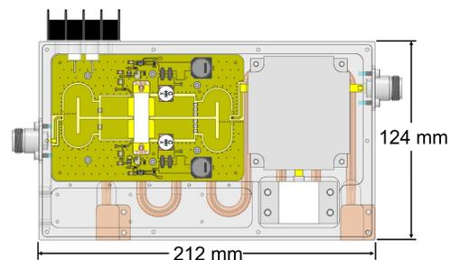
Figure 1: Top view of the amplifier module mechanical assembly CAD.
