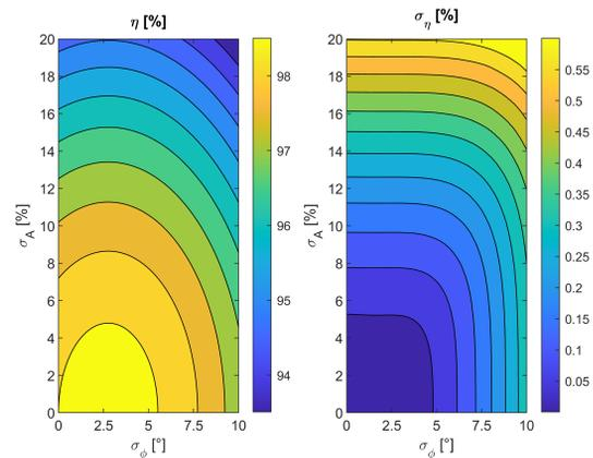
Figure 4: CaCo mean efficiency (left) and its standard deviation (right) for sets of sampled input waves.
