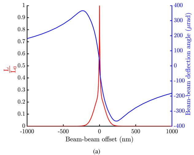
Figure 2: Normalised luminosity (red) and deflection angle (blue) vs. relative vertical IP offset.
