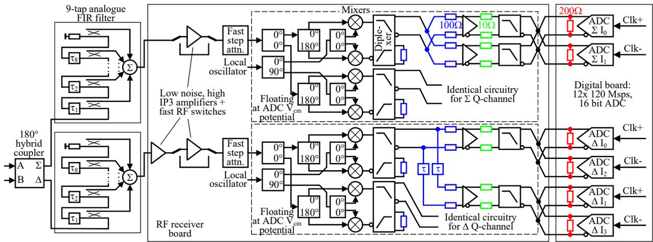
Figure 1: Diagram showing the new receiver topology, with important sub-circuits which influence the overall noise performance. Black lines are 50  $\Omega$  characteristic impedance, blue elements and lines are 100  $\Omega$ .
