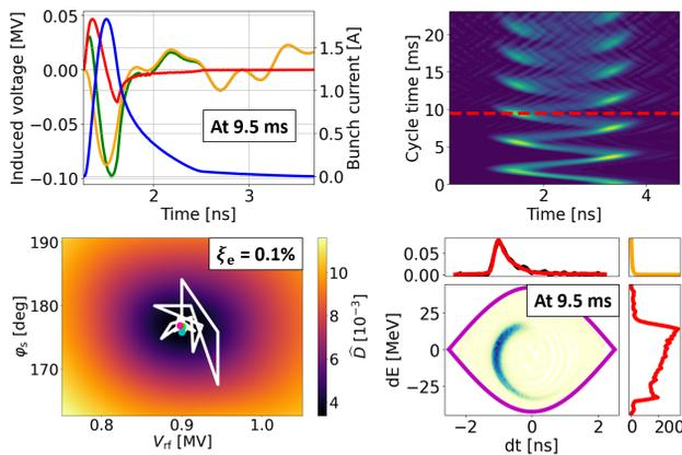
Figure 4: Top left: example of simulated profile (blue) with space-charge (red), impedance (orange) and total (green) induced voltages. Top right: simulated profiles used for voltage calibration. The red line marks the cycle time 9.5 ms. Bottom left: outcome of the voltage calibration. Bottom right: phase-space reconstruction at 9.5 ms.
