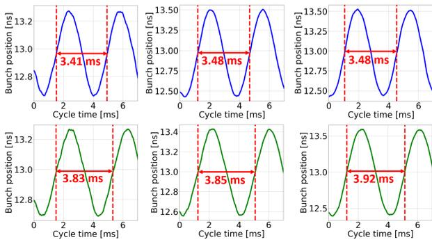
Figure 3: Bunch-position evolutions for cycles measured with only cavity 1 (top) or cavity 5 (bottom), the programmed voltage is 0.9 MV. The bunch positions are the middle points of the profiles FWHM. For each plot, the vertical lines determine one synchrotron period.
