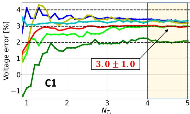
Figure 2: Voltage errors of cavity 1 as a function of the number of synchrotron periods considered for voltage calibrations, using as input the beam measurements taken in October 2021. The results of the five measured cycles are marked with a different color, the red line represents the average. The reported voltage-error average and spread are computed by considering only the data in the shaded area, where convergence is reached.
