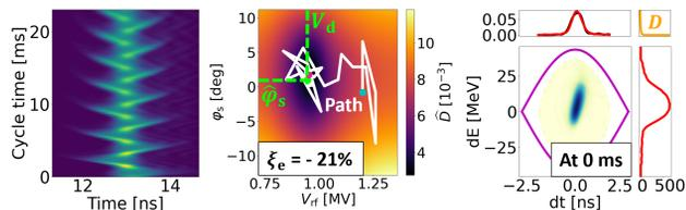
Figure 1: Left: example of bunch profiles measured in 2021 at SPS flat bottom. Only cavity 3 was active with  $V_p = 1.2$  MV. Middle: corresponding voltage calibration. Right: phase-space reconstruction at injection. The measured (black) and reconstructed (red) bunch profiles overlap.
