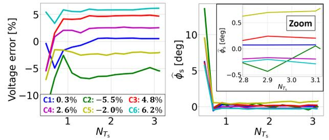
Figure 5: Voltage errors (left) and phase positions of the bucket centers (right) as a function of the number of synchrotron periods used for voltage calibrations. The measurements were taken in early 2022 (only one cycle per cavity). The programmed voltage was 1.37 MV (4 sections) for cavities 3 and 6, 0.86 MV (3 sections) for the other cavities. The voltage errors at  $N_{T_s} = 3$  are reported in the legend.
