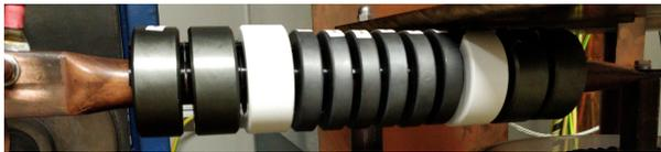
Figure 5: Ferrite cores (2xN87, 1xMat. 43, 6x3C90, 1xMat. 43, 2xN87) consisting of three different materials and sizes.
