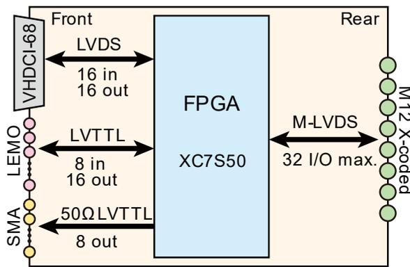
Figure 3: Block diagram of the level converter.
