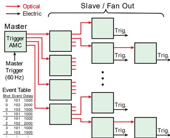
Figure 1: Schematic diagram of the trigger signal distribution system.
