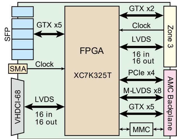
Figure 2: Block diagram of the trigger AMC.
