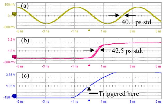
Figure 4: Oscilloscope waveforms from the timing jitter measurement. The external 238 MHz clock is shown in (a), and the trigger outputs from the slave and master AMCs are shown in (b) and (c), respectively. The oscilloscope was triggered by the rising edge of the trigger output from the master AMC (c).
