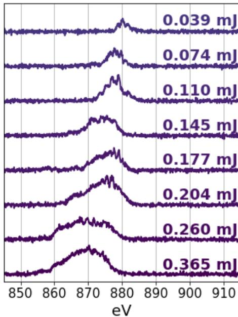
Figure 2: Example spectra are shown for shots with different pulse energies. The highest energy shots have sufficient bandwidth for generation of sub-femtosecond pulses.
