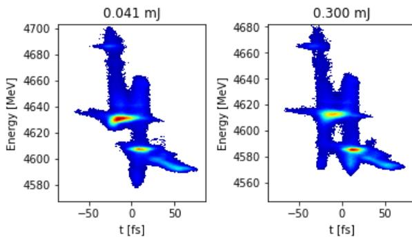
Figure 3: Electron bunch time-energy phase space distribution after the undulators. Energy loss from reamplification in the second stage is seen as the lasing spike in the head of the beam (head on the left).
