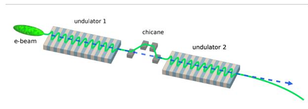
Figure 1: Schematic of the two-stage cascade.
