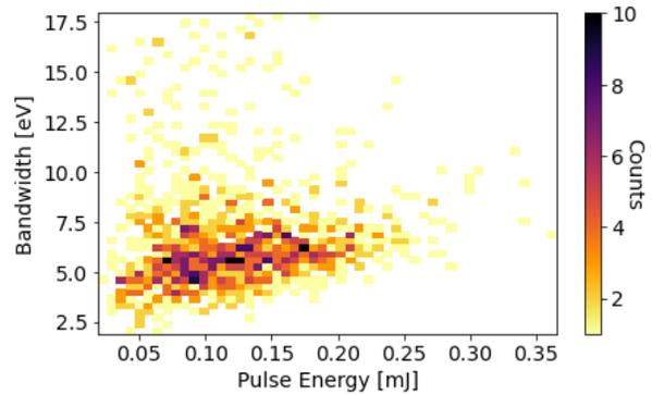
Figure 4: Distribution of bandwidth and pulse energies. The broadening of bandwidth with pulse energy is characteristic of superradiant lasing.
