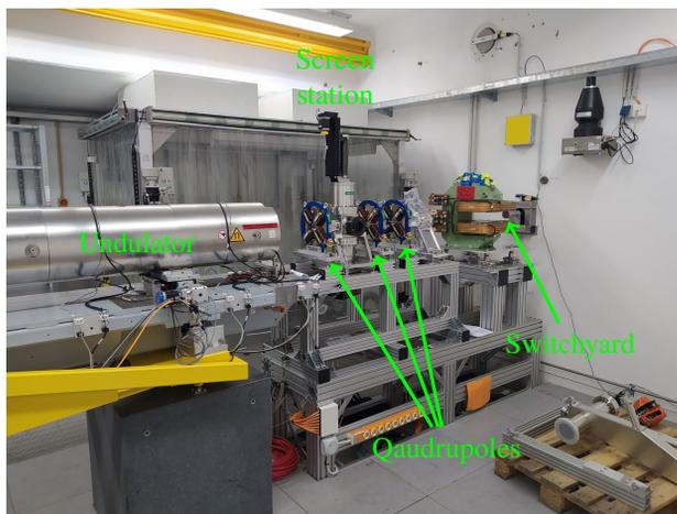
Figure 3: Most of the beam line elements in front of the undulator are installed and aligned. The switchyard magnet support frame was modified and will be aligned shortly and after that the missing bellows and beam tubes to connect the beam line to the undulator vacuum chamber can be installed.
