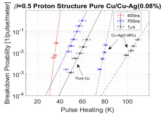
Figure 6: Breakdown rates as a function of peak pulse heating during the pulse.
