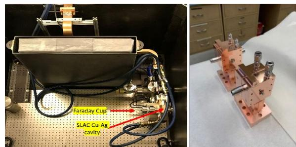
Figure 1: A photograph of the two  $\beta=0.5$  accelerator cavities fabricated at SLAC (right). A photograph of the copper cavity installed on the test stand for high gradient testing (left)
