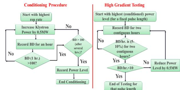
Figure 2: Conditioning and high gradient testing procedure for SLAC copper and copper silver cavities.
