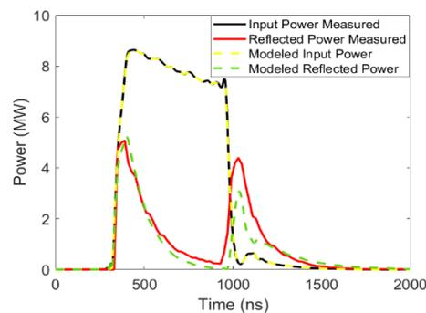
Figure 3: Typical measured 700 ns pulse shape for high gradient testing of SLAC copper and copper-silver cavity.
