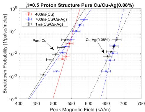
Figure 5: Breakdown probabilities in copper and copper-silver cavities plotted versus peak magnetic field.
