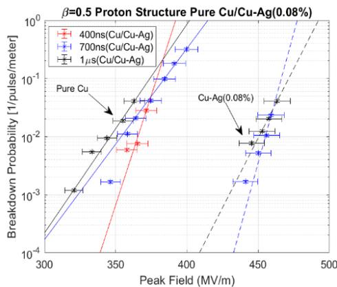
Figure 4: Breakdown probabilities in copper and copper-silver cavities plotted versus peak electric field.
