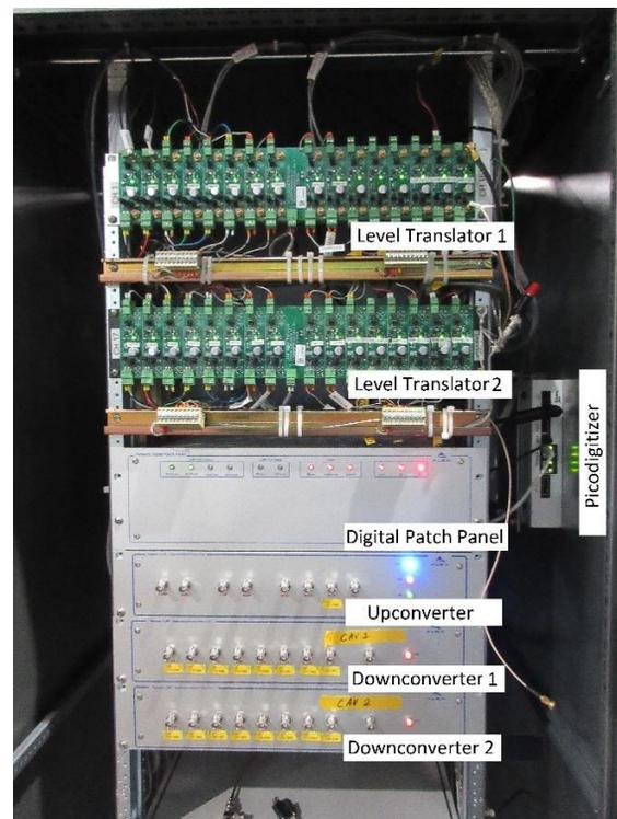
Figure 1: DLLRF components inside the EMI rack.
