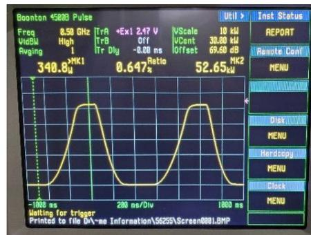
Figure 5: Booster ramping. Yellow: RF envelope.
