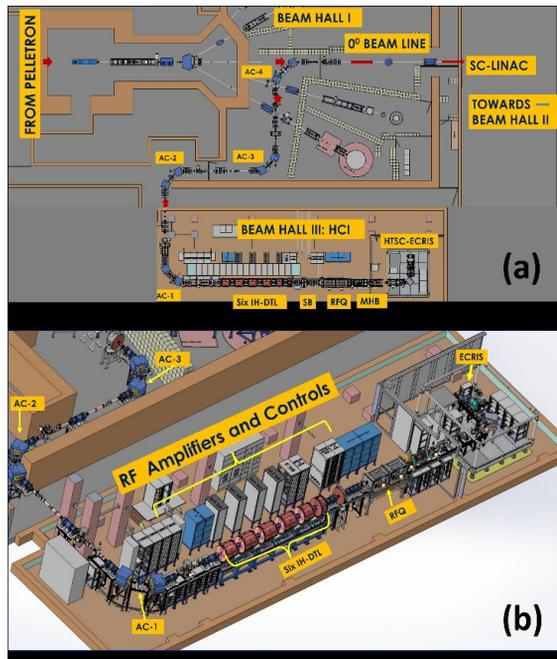
Figure 1: Schematics of (a) HCI design and (b) 3D layout.
