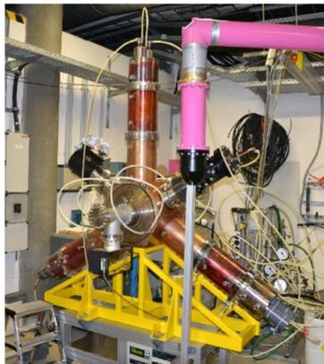
Figure 6: 500 MHz HOM BESSY-type damped cavity.
