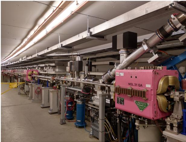
Figure 2: Dipole magnet and front-end components of the dipole beam P66 in the PETRA III tunnel.
