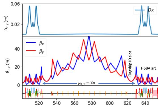
Figure 3: A long straight section featuring 10 m long low-beta insertions for the flagship IDs (north straight).
