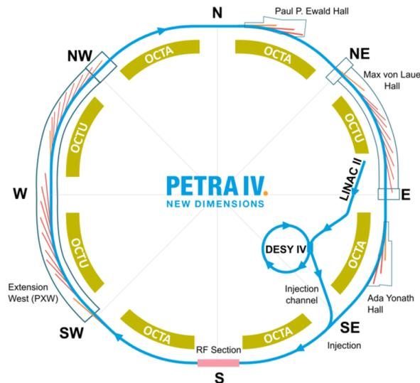
Figure 1: Layout of the PETRA IV facility. Existing experimental halls (Max von Laue, Peter P. Ewald, and Ada Yonath) will be reused. An additional experimental hall ("Extension West") will be constructed.
