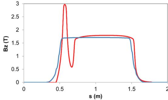
Figure 2: Longitudinal magnetic field profile of the super-bend (red) and nominal dipole (blue).
