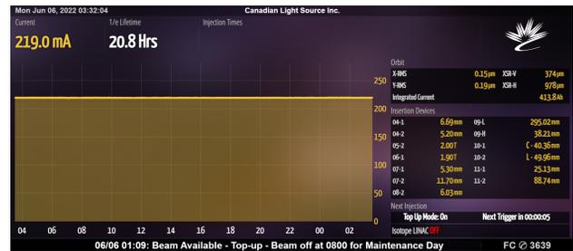
Figure 2: Typical 24 hours of user top-up mode.
