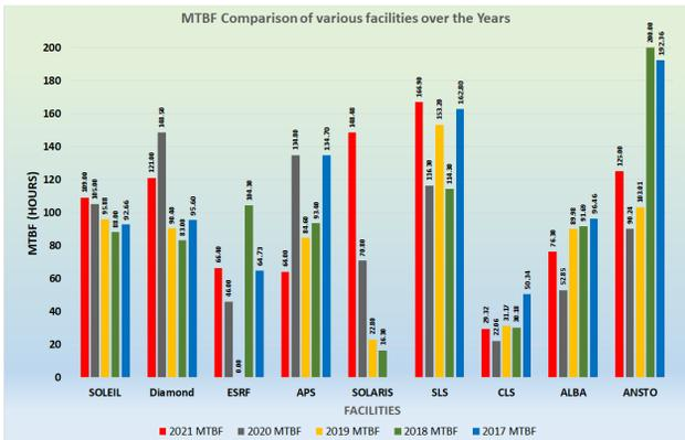
Figure 5: CLS MTBF compared to selected labs.
