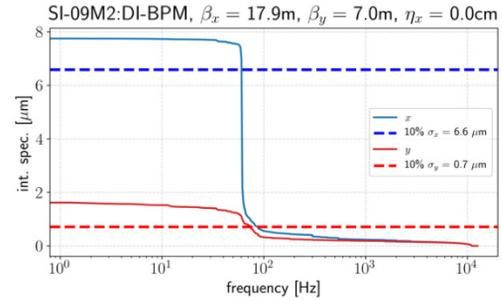
Figure 4: Integrated spectrum from BPM data acquired at 25 kHz sampling rate. The dashed lines represent the requirement of 10% of beam size.
