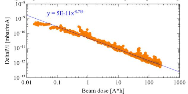
Figure 6: Normalized average dynamic pressure rise ( $\Delta P/I$ ) as a function of the beam dose.
