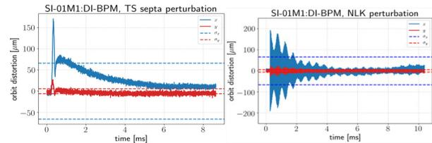
Figure 5: Stored beam orbit transient perturbation due to septa leak field (left) and nonlinear kicker (right). Dashed lines indicate one rms beam size.
