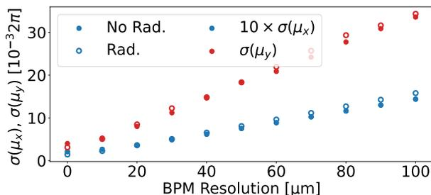
Figure 3: Impact of BPM resolution on horizontal (blue) and vertical (red) rms phase advance error at Z-pole for single kicks (No Rad.) and continuous excitation at the natural tune (Rad.) at  $6\sigma_{x,y}$  using 500 turns for optics measurements.
