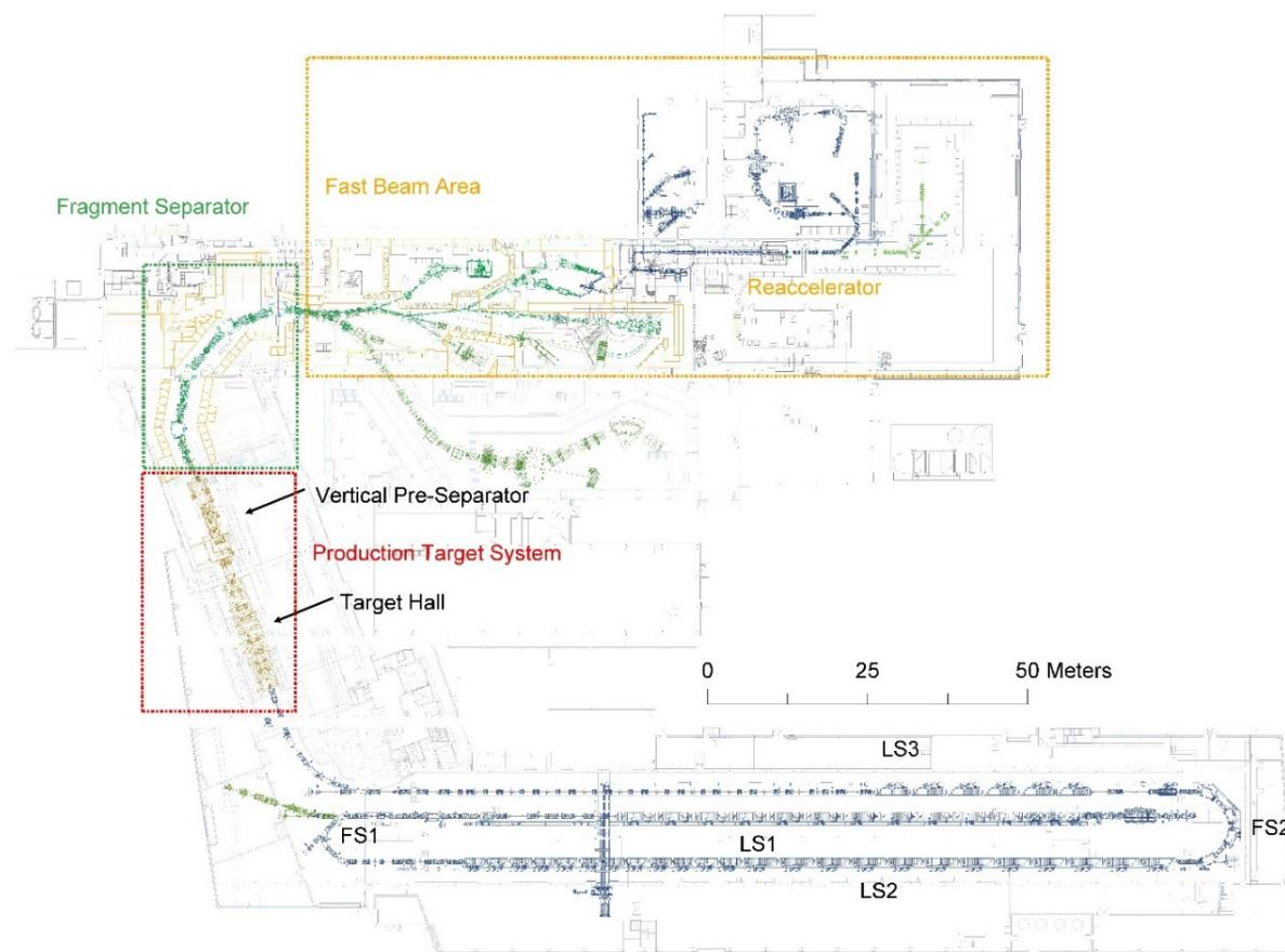
Figure 1: Layout of the FRIB facility. The underground driver linac consists of three straight segments, Linac Segment 1 through Linac Segment 3 (LS1, LS2, LS3), and two folding segments (FS1, FS2), with charge stripping in FS1. The beam delivery system (BDS) delivers beam to the Target Hall at the linac elevation. The vertical pre-separator takes isotope beams to the ground level for transport through the fragment separator to the experimental areas.
