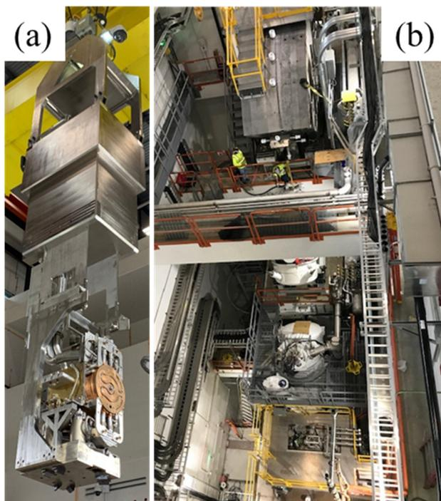
Figure 5: (a) Production target assembly before installation. (b) Vertical pre-separator area.
