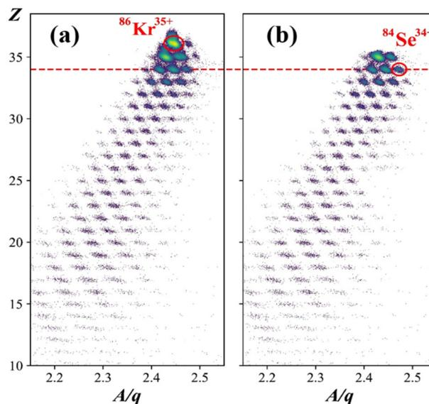
Figure 6: Particle identification for nuclei produced by a  $^{86}\text{Kr}^{35+}$  beam in a 3.3 mm-thick Be target with selection by upstream ARIS magnets: (a) without charge state selection; red circle: charge state +35 of the primary beam, the most intense component; (b) showing only fully stripped ions, as determined by the measured total kinetic energy; red circle:  $^{84}\text{Se}^{34+}$ , the desired isotope.
