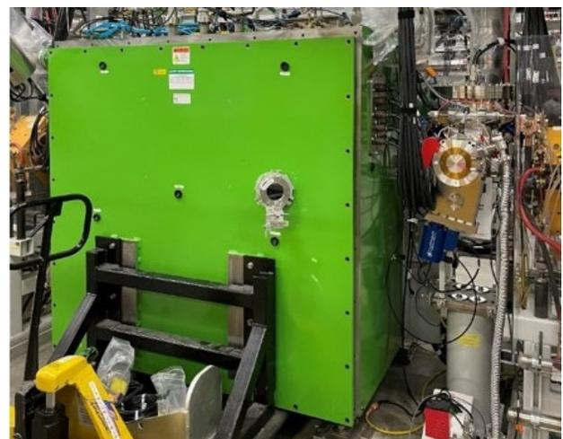
Figure 3: The liquid lithium charge stripper (left) and carbon charge stripper (right) in FS1. The green box is a secondary containment vessel enclosing the entire Li loop.
