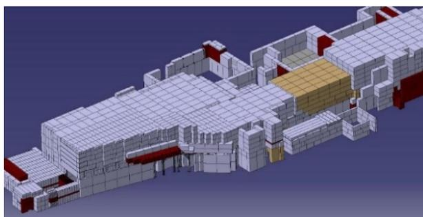
Figure 6: 3D model of the new radiation shield (10.000 t).
