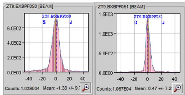
Figure 5: T09 beam profiles on the scintillating fibre detectors in the horizontal (left) and vertical (right) planes.
