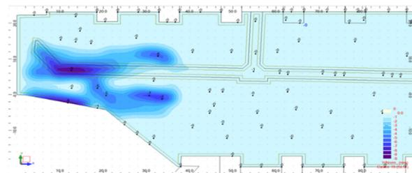
Figure 7: Simulation of the slab deformations (mm).
