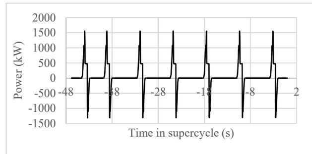
Figure 8: Total output power of all power converters in transfer line F61, F62, F63 and T08.
