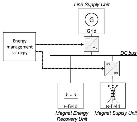
Figure 2: In a Sirius converter energy is being exchanged via a dc-link among three units; the grid-supply, the energy storage and the magnet supply.
