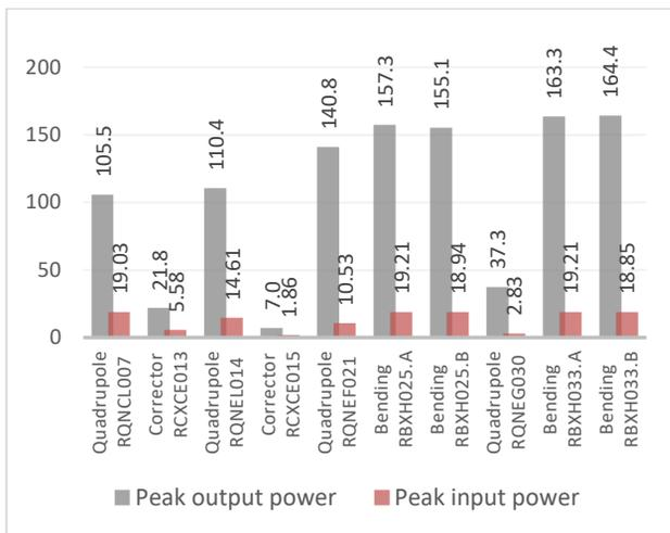
Figure 6: An important difference between the peak input and peak output power of power converters in F61 transfer line of East Area.
