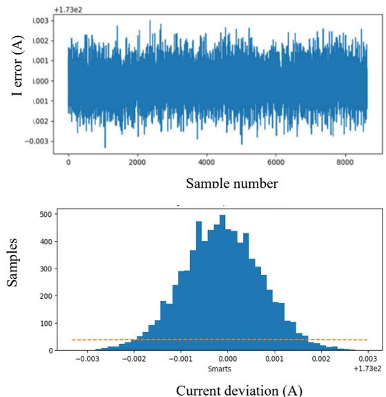
Figure 5: Output current value variation recorded over a period of 24hours. During the magnet current was set to 173A and a deviation of +/-0.003A was recorded that corresponds to 5ppm.
