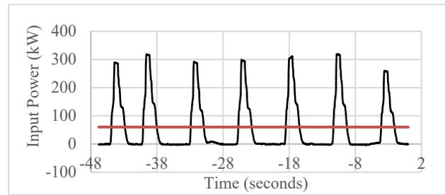
Figure 7: Total input power of all power converters in transfer lines F61, F62, F63 and T08.
