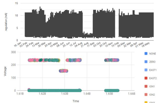
Figure 4: Data from a power converter in TT2 powering a large bending magnet (F16.RBHZ117). Top graph illustrates the evolution of the maximum regulation error over time. The bottom plot illustrates the energy storage state-of-charge (voltage) as a function of time for different users.
