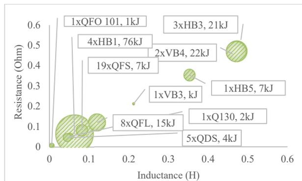
Figure 1: Inductance and resistance value of the magnet loads in the TT2 transfer line. Bubble size corresponds to the energy stored by the magnet.
