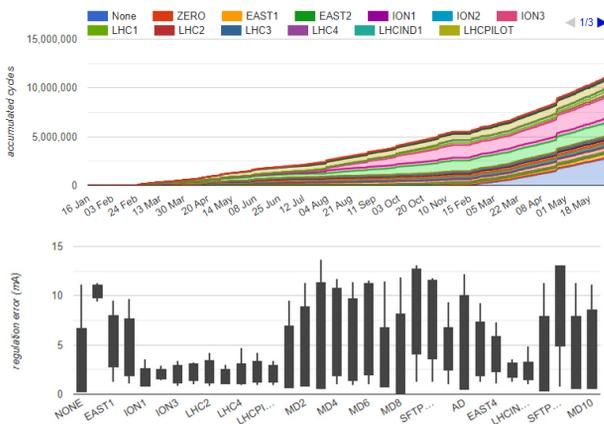
Figure 3: Data from a power converter in TT2 powering a large bending magnet (F16.RBHZ117). Top graph illustrates the accumulated number of cycles played for different accelerator users in present year and the bottom plot shows the spread of regulation precision for different accelerator users (67% of samples are within boxed area).
